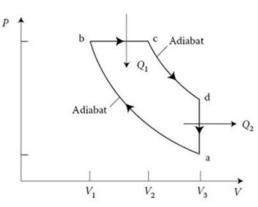
7) Which of the following expressions defines the *efficiency* of this engine, if W represents the net work done by the gas in one cycle?
